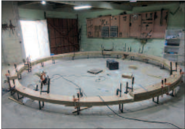
Two more arcs to add to make up the second layer. Mike will machine the outside surface, then the wrought-iron band can be fitted. Then the inside surface must be machined very accurately round. He must then make another ring which rotates inside this curb, which will be fixed down on the tower with the studs.
