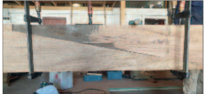
One of Jon's scarfs in the massive sheers, made from old Bilinga wood which he had.
