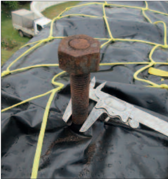
The studs on the top of the tower are 3/4in diameter. I will have two discs machined to make measurements more accurate.
