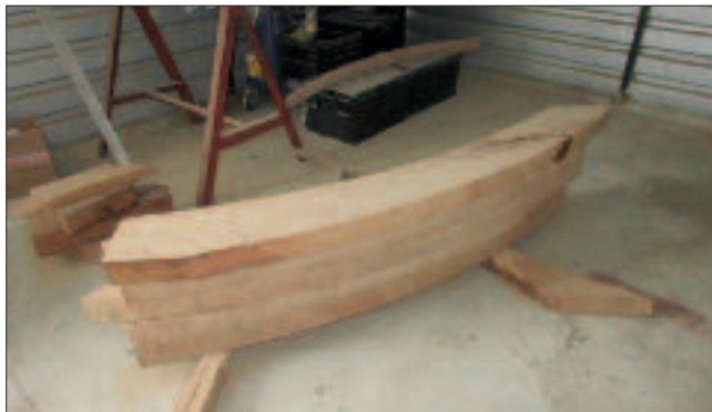
Some of the segments of the curb rings which Mike has been cutting.
