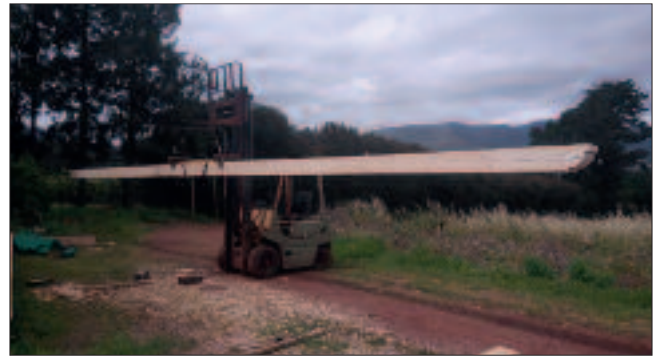
This is the long stretcher which I've made, hanging from the forklift in the middle. It's spruce, 12m long and 200mm square.
