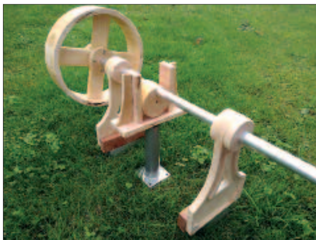
Wooden pattern for the cast parts of the feeder.
