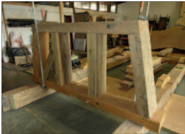
The Dutch call this 'Het voorkeuvelens', the front gable, perhaps? The middle two uprights which will hold the neck bearing in place are Stinkwood! Jon made it as if it was going to stand vertical, but it must lie over at 10 degrees, so he will deepen the dovetails be's made in the sheers and Burgemeester at the front.
