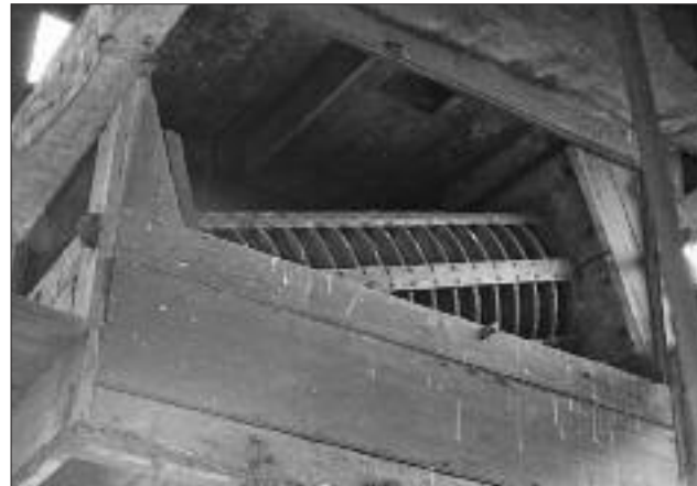
The Pitstone dresser when installed at Chinnor (left) and the possible vibratory feeder (right).
