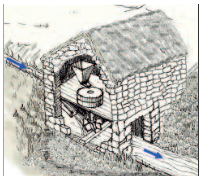
Fig. 2. Representation of a typical Shetland horizontal mill. Part of the gable end wall has been removed in the drawing to show the milling mechanism inside.
