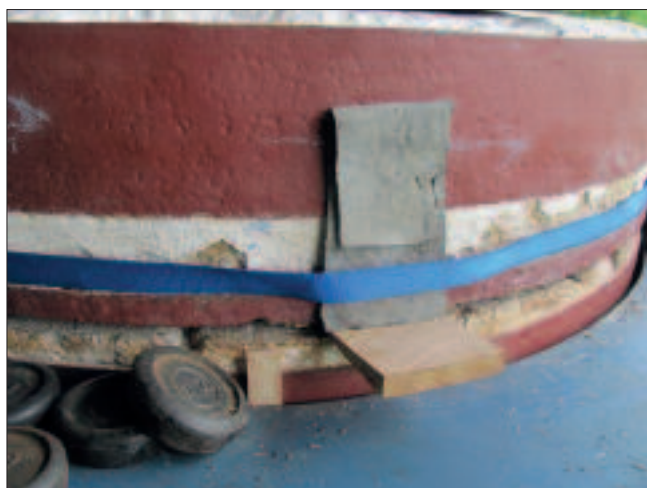
Using sheet lead and strapping to identify balance points.
