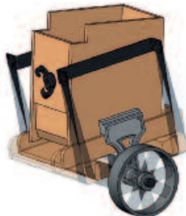
Illustration of the vibratory feeding movement of the chute oscillating on its four supporting leaf springs, created by the pulley-driven eccentric.
