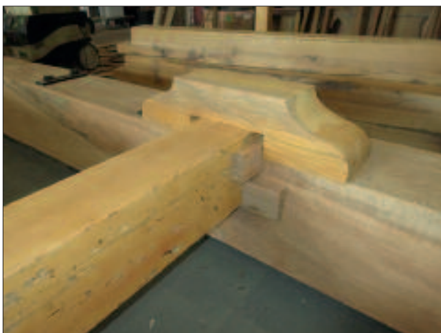
The bridges have been made to hold the sprattle beam, which must also be able to move laterally and fore-and-aft, by adjusting the wedges.
