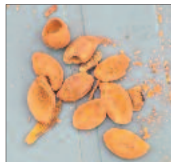
Some of the nuts retrieved from the radiator and engine block.
