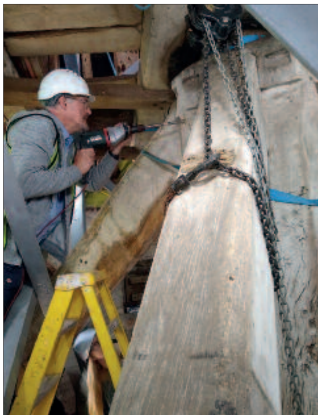
Martin Bridge drilling the core taken from the main post. Picture – David Holmes.
