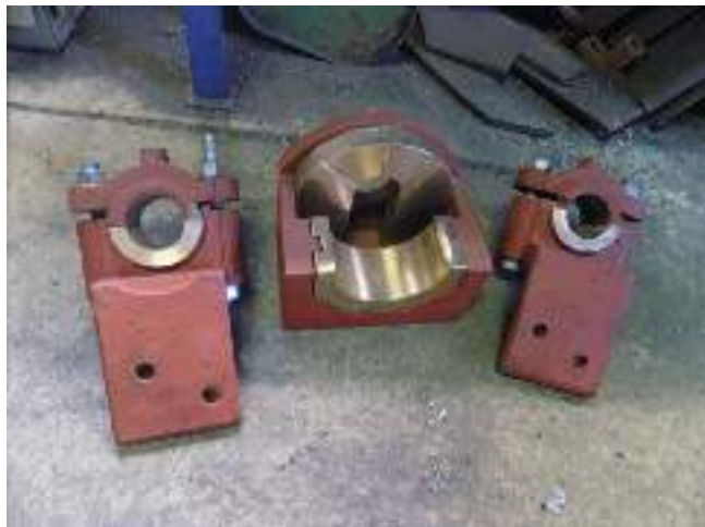
Fly spindle plummer blocks/angle bracket, new windshaft tail bearing assembly.
