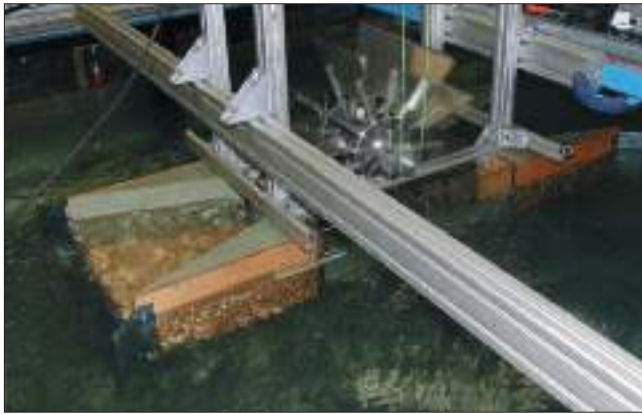
Fig.4. (a) The floating water wheel with the hydrodynamically shaped floating structure, that can convey water to the wheel with minimum head loss (experimental installation, W.M.J. Batten Batten et al. (2011)); (b) example of a floating wheel in deep water, real installation (photo of Salmini Santino Elettromeccanica, Italy)
