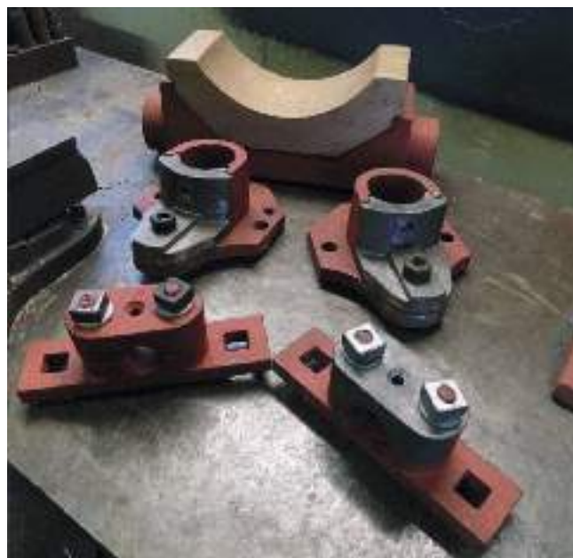
New neck bronze, new keeps (worm spindle bearing cups) re-machined y-wheel spindle bearings
