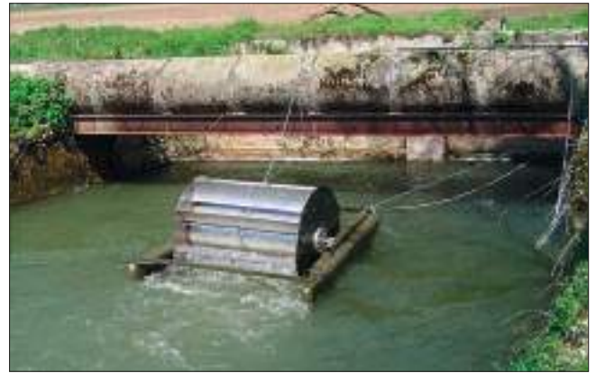
Fig.4. (a) The floating water wheel with the hydrodynamically shaped floating structure, that can convey water to the wheel with minimum head loss (experimental installation, W.M.J. Batten Batten et al. (2011)); (b) example of a floating wheel in deep water, real installation (photo of Salmini Santino Elettromeccanica, Italy)
