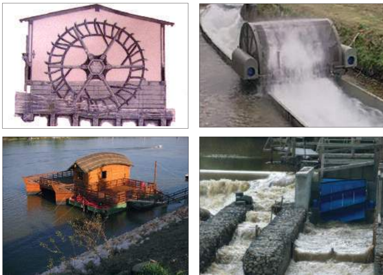
Fig. 3. Stream water wheels in: (a) subcritical shallow flow, (b) supercritical shallow flow (photo of Emanuele Quaranta), deep flow (photo courtesy of AIAMS Italy) (c), and Hydrostatic Pressure Machine (picture of Nick Linton) with diagonal blades to reduce water resistance (drag forces) at the blades (described in Innovations section) (d).
