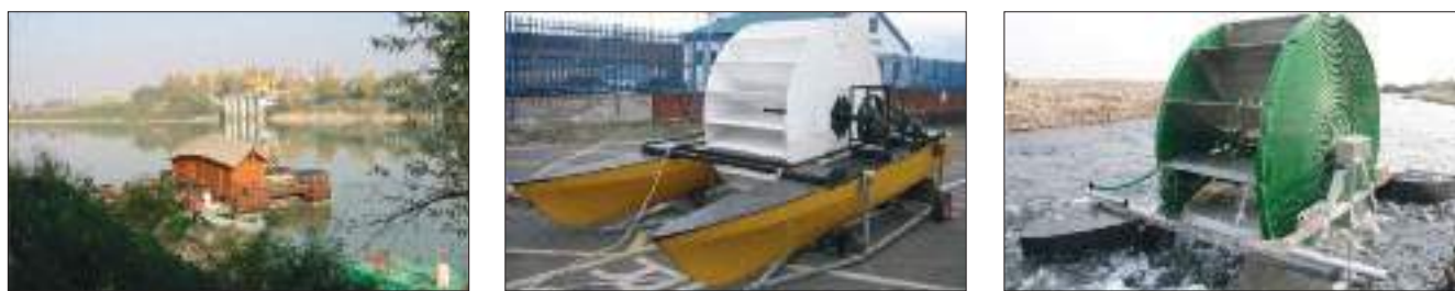
Fig.2. Stream water wheels for different purposes: (a) mechanical power generation (photo courtesy of AIAMS Italy), (b) electricity production (Turnock et al., 2007), and (c) pumping in irrigation systems (photo courtesy of Jaime Michavila (Aqysta)), see Quaranta (2018).
