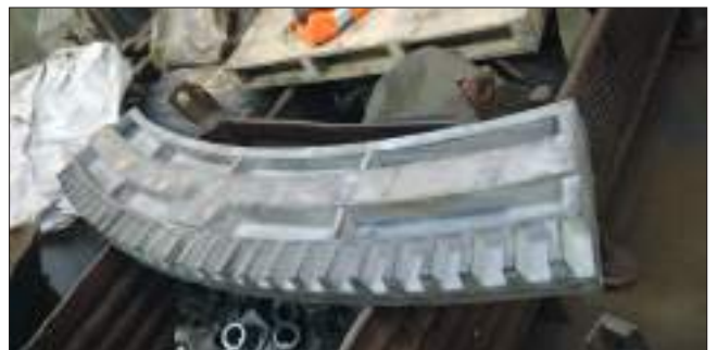
Pouring molten iron into the mould for the segments of the curb, at Boro' Foundry in Stourbridge; a segment of the raw cast curb; and the cast-iron cross emerging from the sand at H. Downs of Sheffield.
