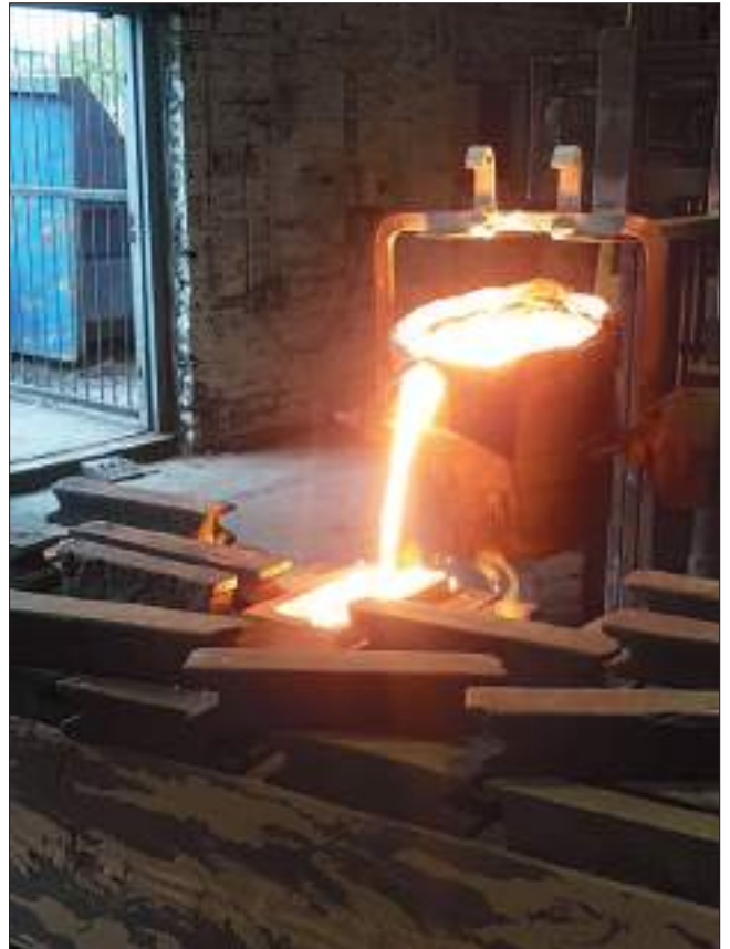
Pouring molten iron into the mould for the segments of the curb, at Boro' Foundry in Stourbridge; a segment of the raw cast curb; and the cast-iron cross emerging from the sand at H. Downs of Sheffield.
