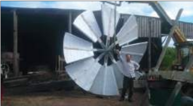
The new cast-iron windshaft and cross, and the new fantail, at Adam Marriott's workshop.
