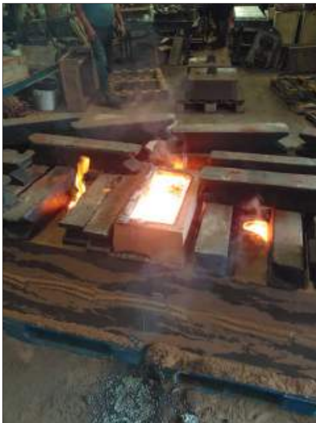
Pouring molten iron into the mould for the segments of the curb, at Boro' Foundry in Stourbridge; a segment of the raw cast curb; and the cast-iron cross emerging from the sand at H. Downs of Sheffield.
