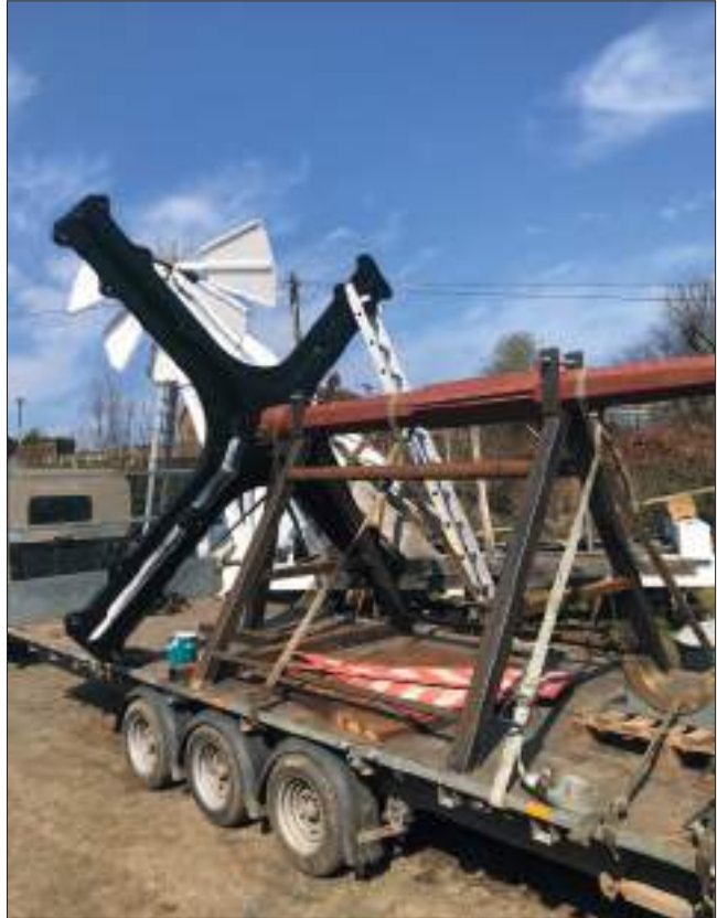
The new cast-iron windshaft and cross, and the new fantail, at Adam Marriott's workshop.
