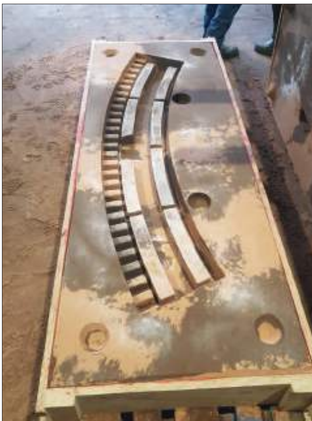
Making the pattern and casting mould for the segments of the curb.
