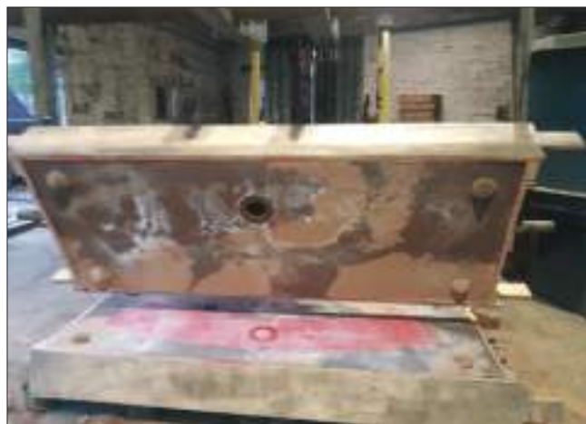
Making the pattern and casting mould for the segments of the curb.
