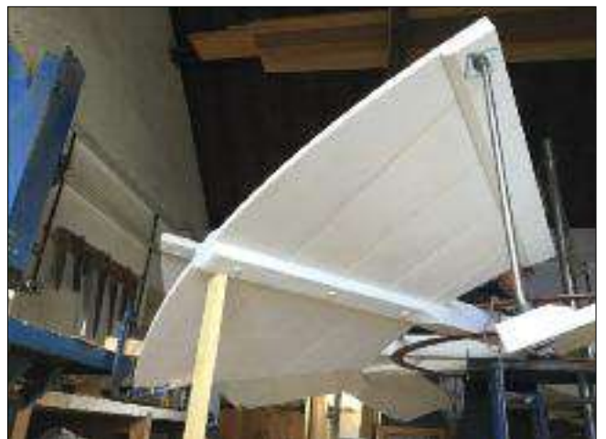
Detail of fly blade and tip tie rod.
