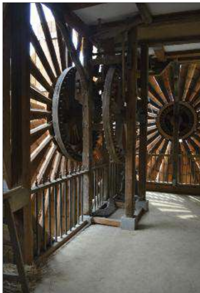
Interior of the barn mill at Saalow showing the two annular wind wheels. Picture – Graham Hackney .
