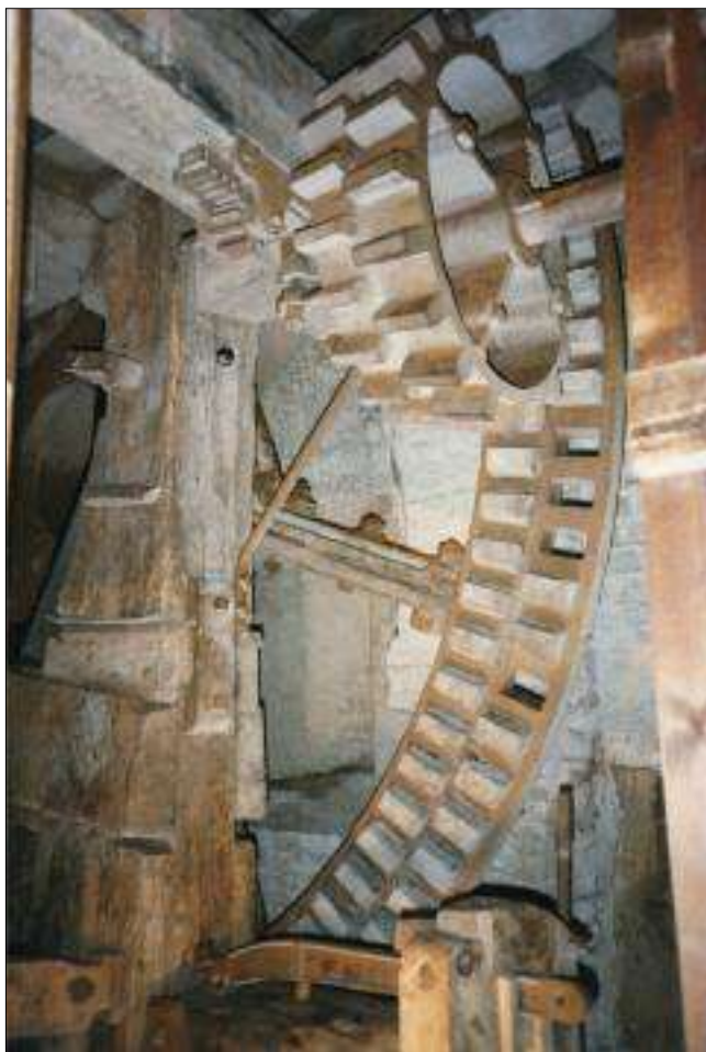
Double-cogged pit wheel at Houghton Watermill. Picture – Hampshiremills.org .
