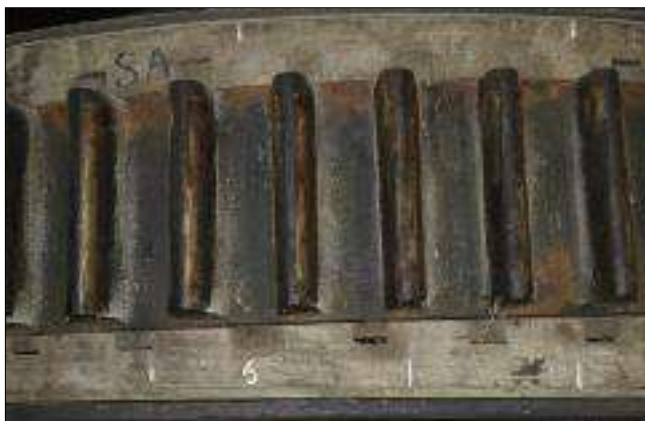
Staggered double cogs at Heage Windmill, the tenons clearly evidenced behind the later single cog iron sections.
