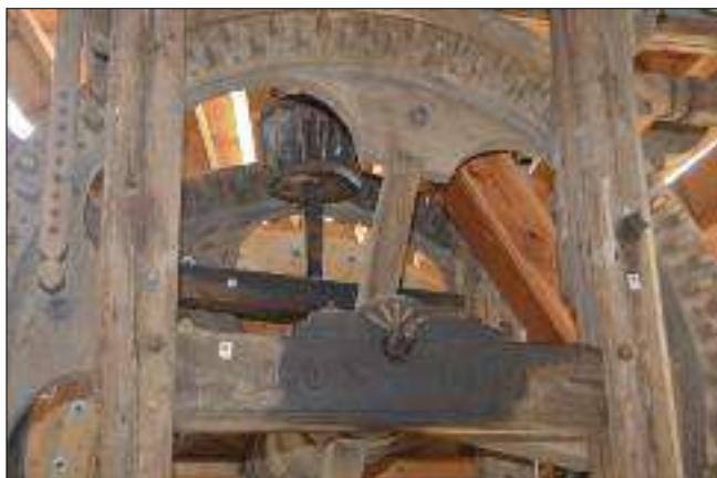
The two brake wheels at Saalow; both are double-cogged and the outermost wheel still has its lantern gear.
