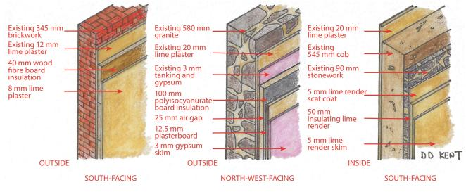
In-depth assessment was made according to a number of parameters both before and after work aimed at thermally upgrading several solid walls of varying construction using a range of methods and materials (not necessarily advocated by the SPAB). Illustration: Douglas Kent
