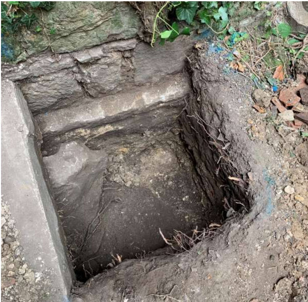
Figure 10: TP5 looking north-west with the in situ and disturbed Gault Formation at the base of the pit, overlain by the offset masonry. Note the massive piece of quarry stone on the left edge.
