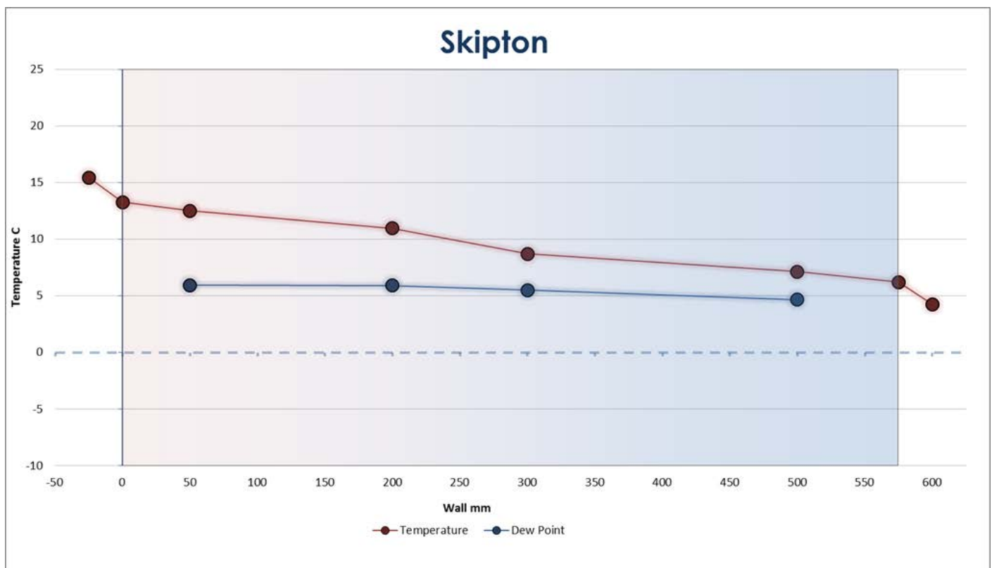
Figure 62: Hygrothermal Section, White House Farm, Skipton, 10th - 24th February 2011.
