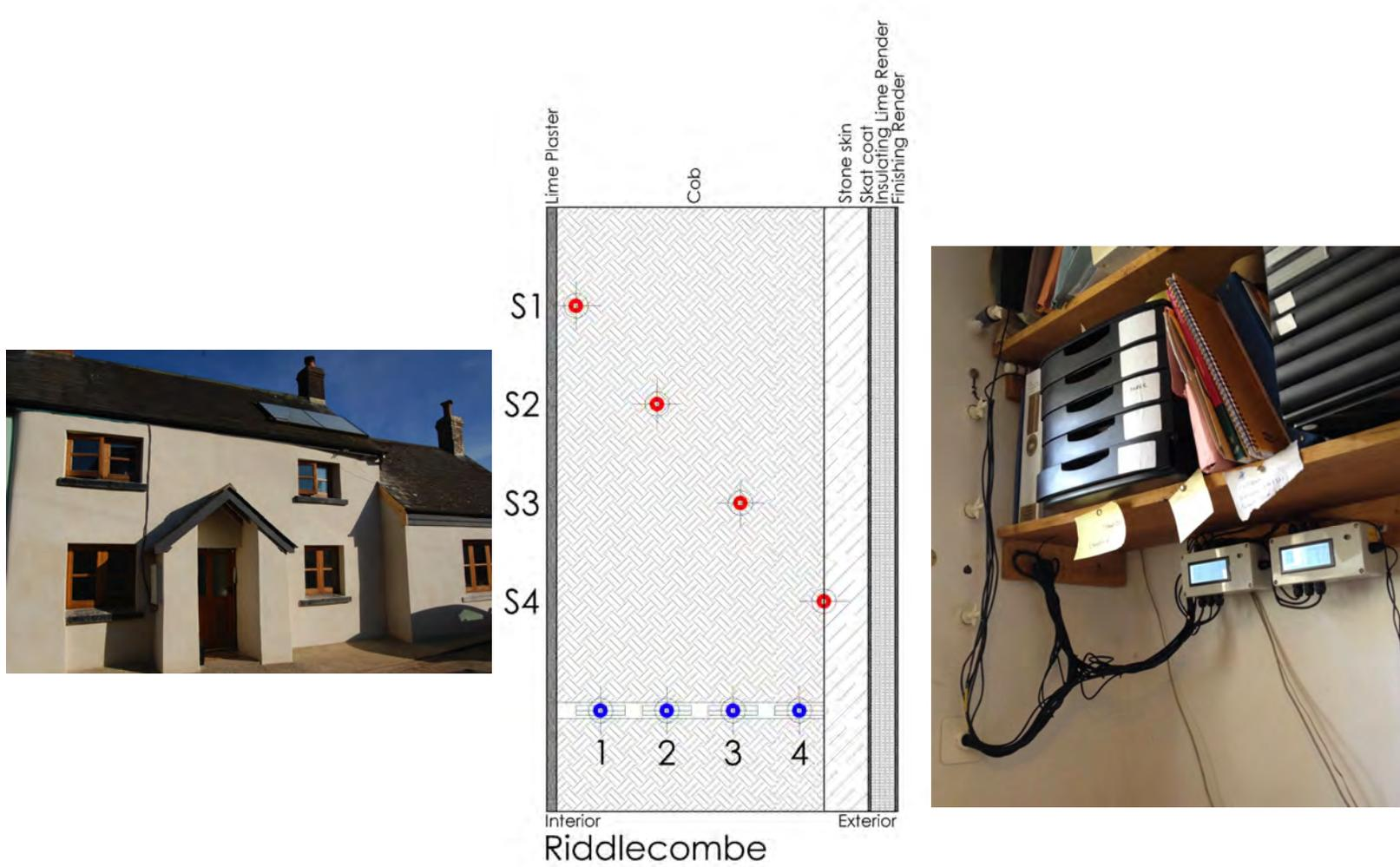
Figure 4. Interstitial hygrothermal gradient and material moisture monitoring, Riddlecombe.
