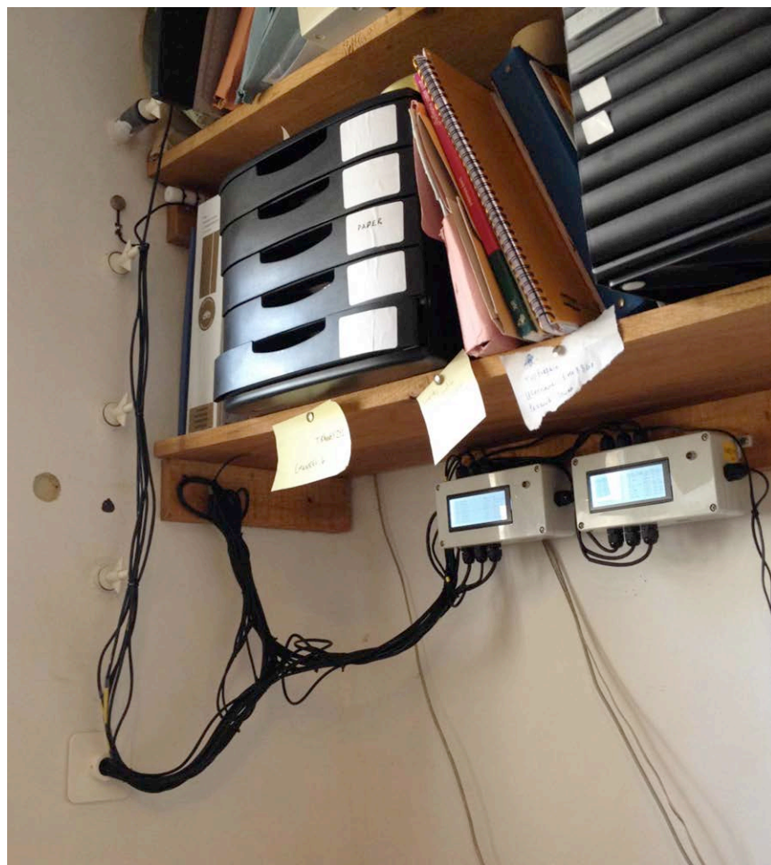
Figure 37. Interstitial hygrothermal gradient and material moisture monitoring, Riddlecombe.
