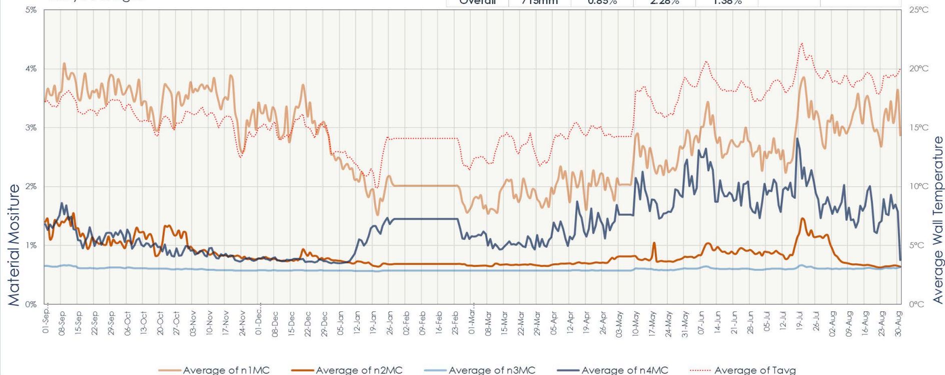
Figure 47. Material moisture content over time, The Firs, Riddlecombe 2015-2016.
