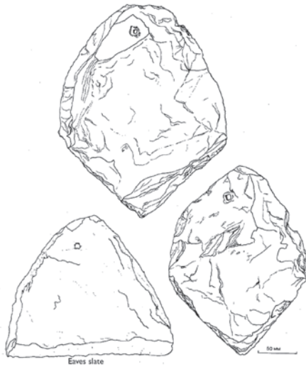
Figure 26 As at other Roman sites the slates are hexagonal. These are often described as diamond shaped or four sided but the actual hexagonal shape is fundamental to the way they are laid to form a water tight roof. McWhirr 9
