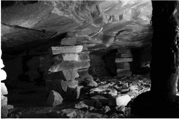
Figure 44 Historically Collyweston log mined by extracting the sand from below and propping the roof using a pick and the roof on temporary pillars until an area about 12 or 15 feet deep had been cleared. The pillars were then removed and the log allowed to fall. Terry Hughes
