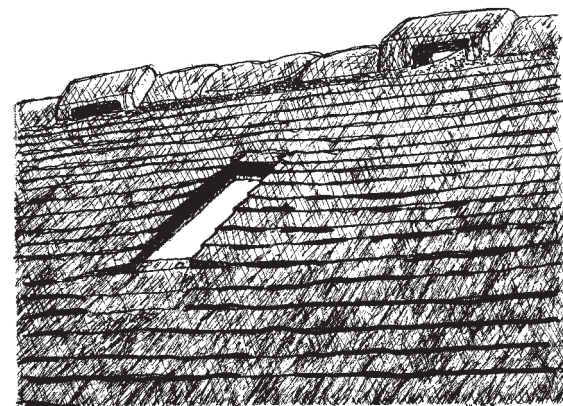
Figure 22a In their simplest form rooflights are just a sheet of glass substituted for a slate or inserted into the slope and the slating overlaid. These are common on farm buildings.
