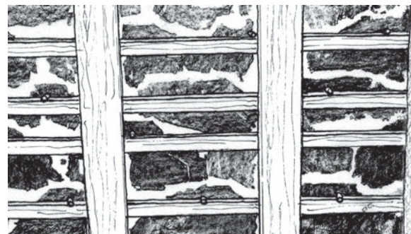
Figure 23b Torching is applied to the underside of the slates and may just cover the top of the slates (single torching) or their backs completely between the laths (full torching).
