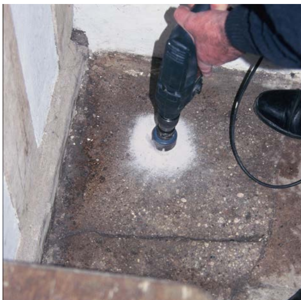
Figure 14: Drilling to remove a core sample of a gypsum plaster floor for laboratory analysis. Photo: A J Goode Ltd
