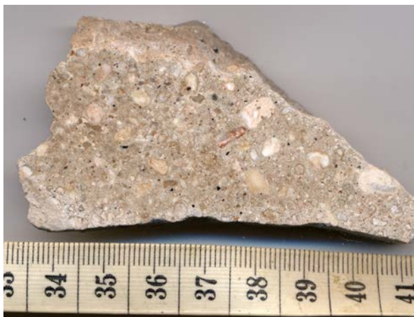
Figure 1(a) Figure 1: Samples of old gypsum plaster floors: (a) typical colour and texture, and; (b) the varied composition found.
