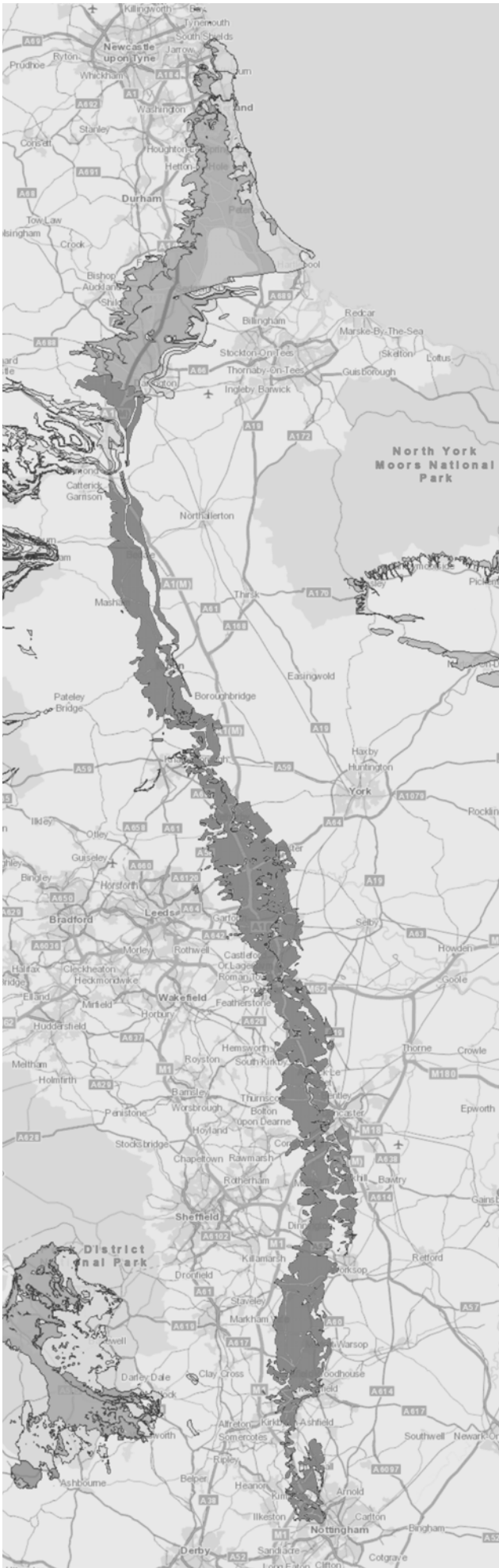
Figure 30: The Magnesian Limestone Formation extends for 150 miles (240 km) from Nottingham to Sunderland, Tyne and Wear. There are only a few roofs with this slate known today, in an area from Mansfield to Doncaster – at Steetley, Barlborough and Whitwell. Image: Reproduced with the permission of the British Geological Survey © UKRI 2019
