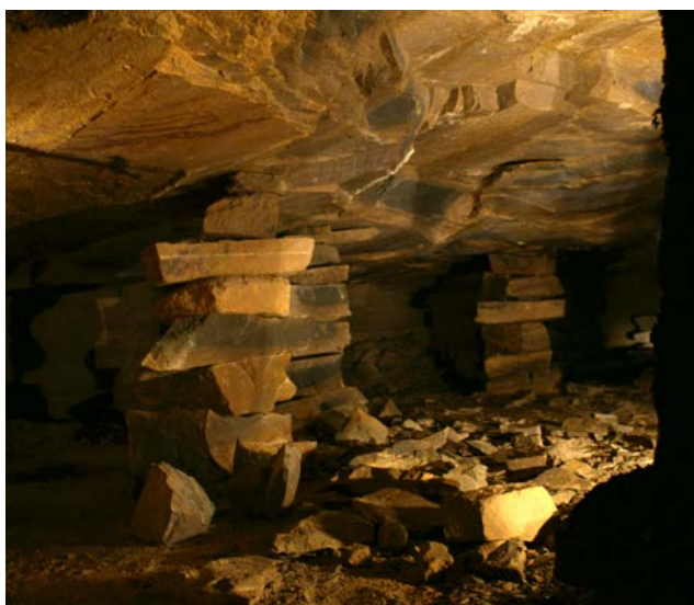
Figure 31: Historically, Collyweston log was mined by extracting the sand from below using a pick and propping the roof on temporary pillars until an area about 12' to 15' (3.5 to 4.5 m) deep had been cleared. The pillars were then removed and the log allowed to fall. Photo: Terry Hughes
