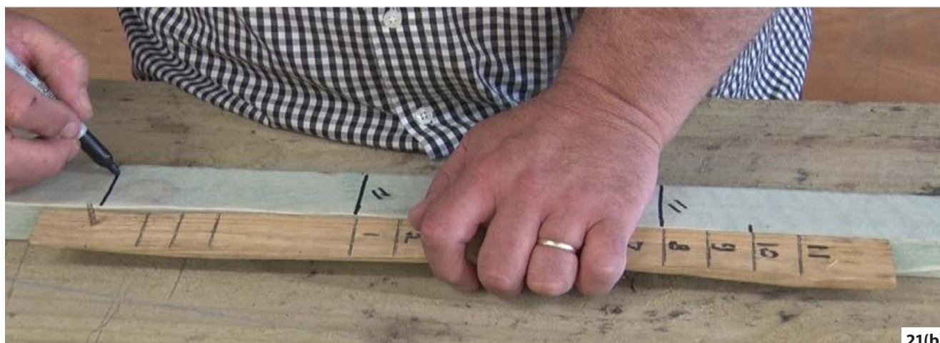
Figure 21: Gauging: (a) Slater's marking sticks vary regionally but all have a mark for each slate length and a pin at one end. The marks can be numbers or symbols and do not necessarily designate inch lengths. Some also include head lap marks – usually 1, 2 and 3" lengths – or lath gauges corresponding to each slate length. (b) The stick is used to set out the margins and the lath gauges and these diminish all the way up the roof.
