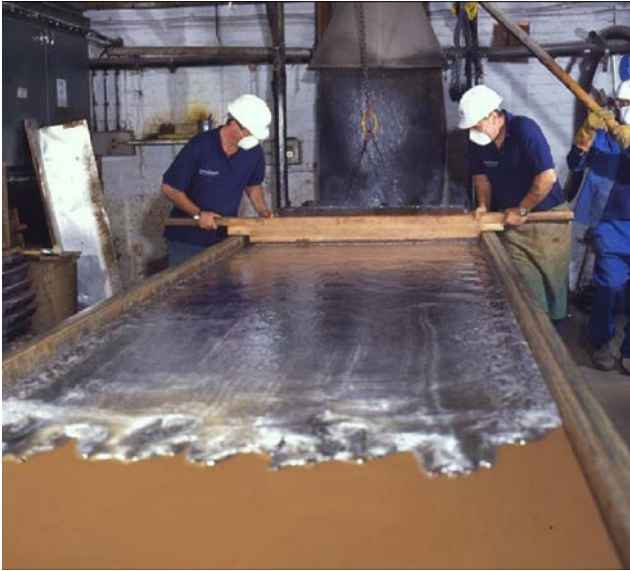
Figure 13: Sand-casting of lead sheet. Photo: Norman & Underwood Group Ltd
