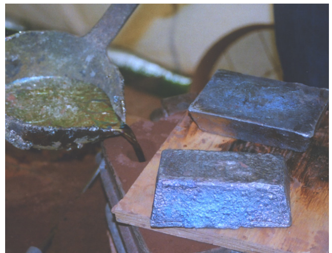
Figure 20: Casting molten lead in a two-piece mould. Photo: Douglas D Kent
