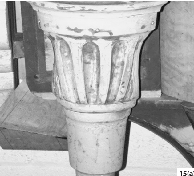
Figure 15: Formation of a decorative rainwater head: (a) Half-round wooden block over which lead is dressed. (b) Half-round 18th-century rainwater head having been dressed over wooden block at 16 Watling Street, Canterbury, Kent. Photos: Peter T J Rumley
