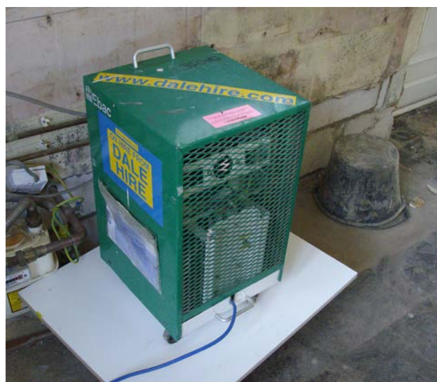
Figure 28: Dehumidifiers are rarely a practical long-term solution for condensation problems. Photo: Douglas Kent
