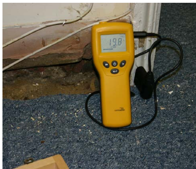
Figure 18: Electrical moisture meters have a role to play in diagnosing problems when used in the correct hands.
