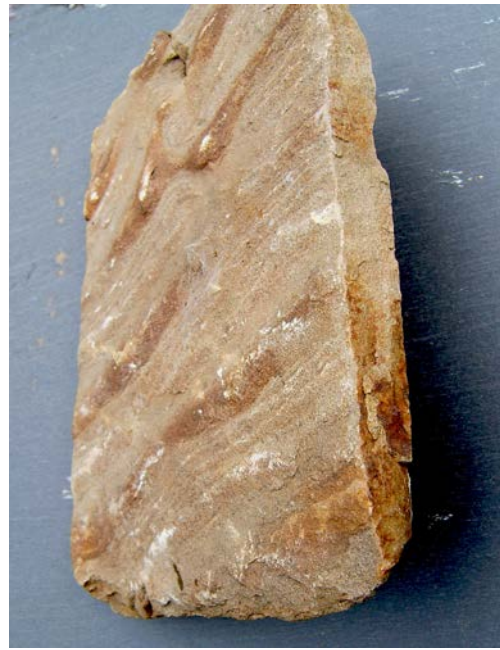
Figure 37. Almost all region's stone slates are sandstones. Pennant sandstone from near Pontardawe.
