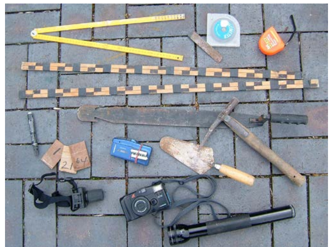
Figure 8. Recording the way a roof was slated can be difficult, perhaps involving several measurements on each of 50 or more courses. Equipment should be chosen to be convenient when working on a roof ladder. Photography and voice recordings will ensure details are not lost or recorded for the wrong course. Also, every slate removed destroys its relationship with the surrounding slates, so if a video recording can be made it allows the stripping to be ‘reversed’ to check the details subsequently.
