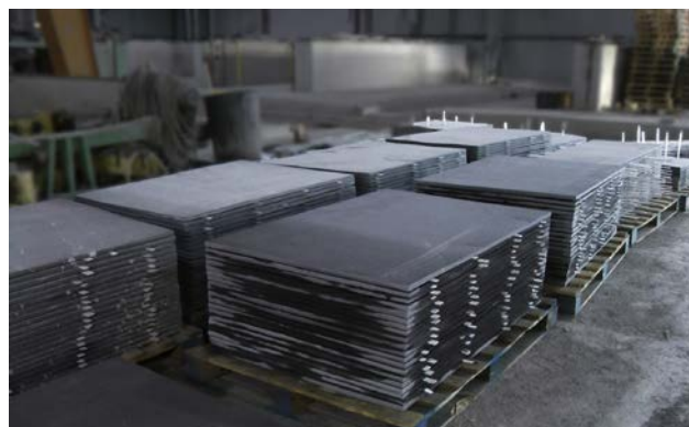
Figure 15. Quarries can make slates to specific sizes or formats given reasonable warning. These slates measuring 1350 x 950 mm were made by Welsh Slate for the Patent slating of St George's church, Everton, Merseyside.
