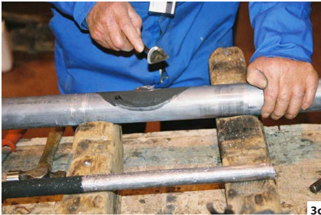
Figure 3: Formation of a branch wiped joint demonstrated on an SPAB course: (a) Opening up to receive the branch pipe. (b) Use of compasses and a scribing plate to incise the line of the joint. (c) Scraping back the masking fluid. (d) Applying the solder. Photos: Douglas D Kent
