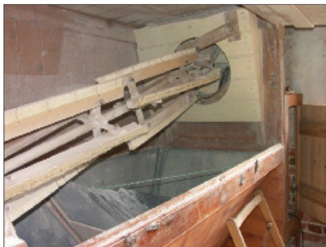
Dressing machine stripped down for cleaning.
