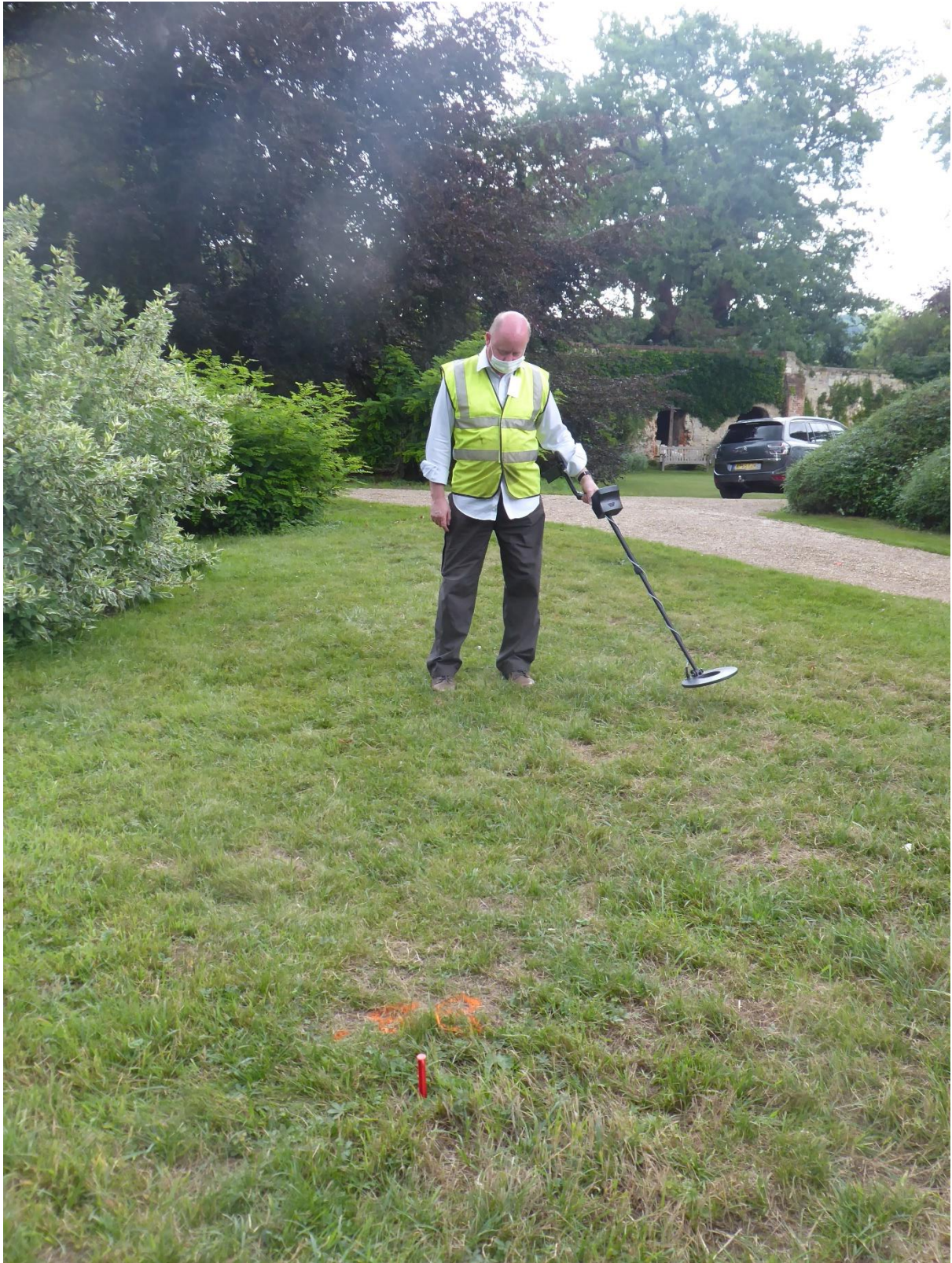
EDC 6 in the foreground. The line back up to EDC 5 is being found (surprisingly effectively) by a metal detector. It broadly heads under, but to the right of the trunk of, the copper beech in the distance and then to the left of the end wall of the terrace.
