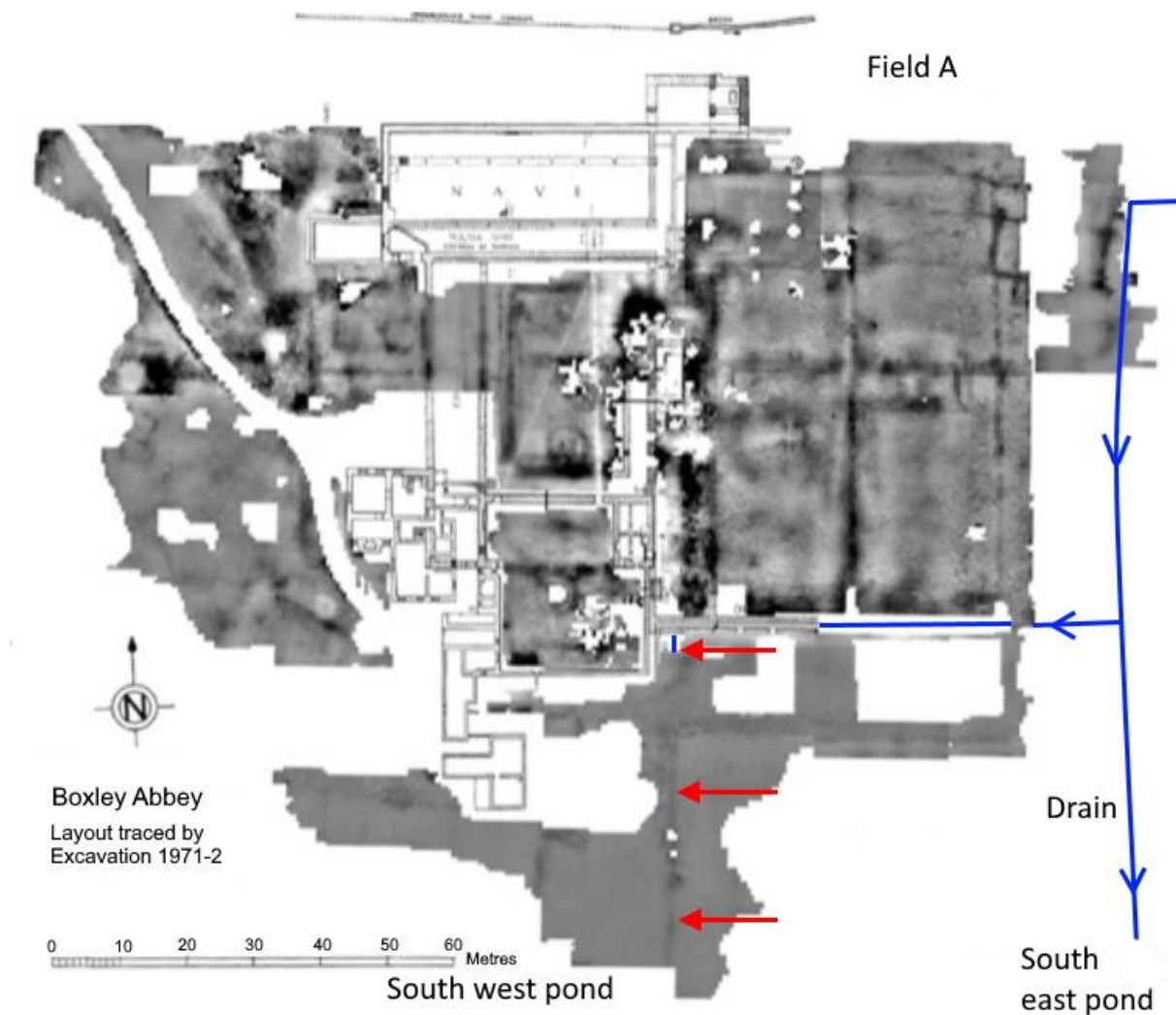
Figure 15 - The grey-scale resistivity survey results within the garden at Boxley Abbey, Kent overlaid on the 1971-2 layout interpretation (Tester 1973, Fig. 1). The reredorter drain is highlighted by the red arrows.
