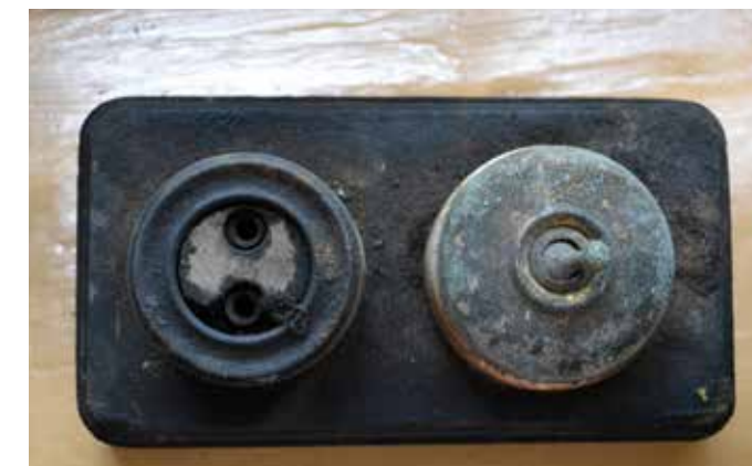
Above Burnt electrical fitting found under floor boards
