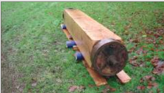
Wrickton Watermill, the new wheel shaft.
